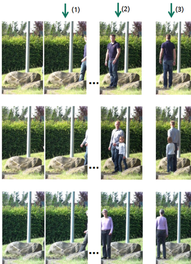
Fig 2: Video sequences of prototypical traffic scenes with key frames for pedestrian detection (1) and recognition of uncritical (2) and critical (3) traffic situations.
